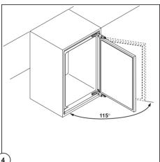
Push the appliance into place and retain the cabinet with screws through the securing brackets into the worktop or adjacent woodwork as necessary.
